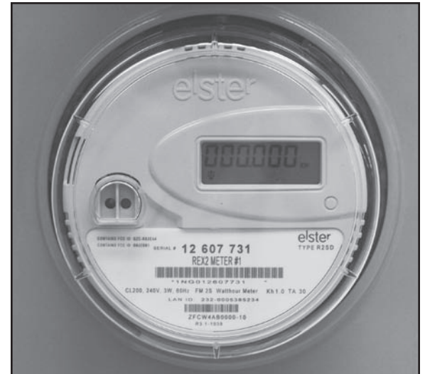
AMI meters look similar to the older electromechanical meters in use across Co-op service territory. Instead of gears and dials, AMI meters use a digital display to measure electric usage. A small transmitter in each meter sends usage data several times a day.
