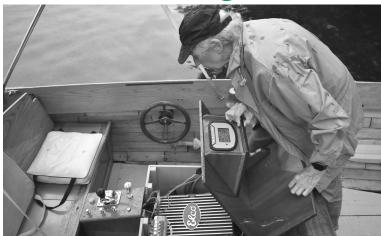
Co-op member Bill Porter of Holderness shows off the power plant in his 1926 Johnson Laker — an eco-friendly, 105-amp electric motor that charges in 3-4 hours, never needs a tune-up and produces no emissions. The motor is virtually silent when operating, allowing Bill and his family to enjoy the tranquility of Squam Lake. Manufactured by Elco Motor Yachts of Athens, NY, the motor has a miles per gallon equivalency of 65 mpg and maximum range of more than 30 nautical miles per charge!
